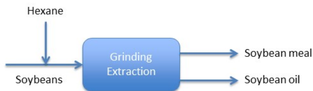
Figure 6: Production steps of soybean meal and soybean oil.
