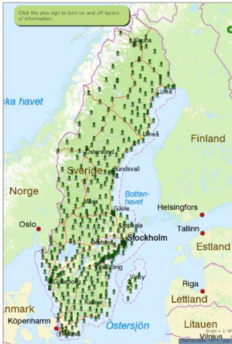
Figure 2.2 SWEPOS stations and other stations used in positioning services (source: https://swepos.lantmateriet.se/tjanster/kartstod/kartstod.aspx ; data accessed: 26 th Feb 2016).
