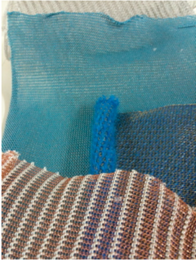
Figure 1 This picture show three conductive textile samples in different knitting stitches. Front: knitted copper with viscose. Center: knitted blue mohair with brass. Back: knitted turquoise cotton with stainless steel. All samples are made at The Swedish School of Textiles on a circular knitting machine by technician Tommy Martinsson
