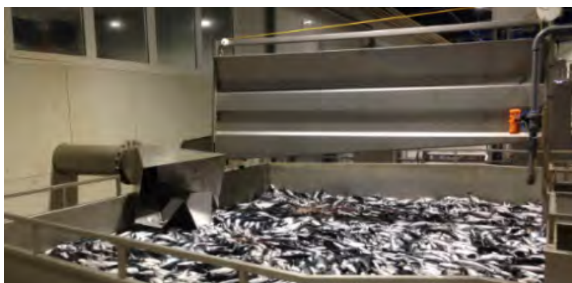
b) The fish including pumping water is pumped into the intake tank.
