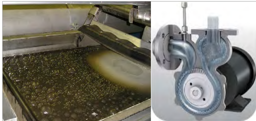
Figure 32. The Micro-DAF flotation system and the Nikuni pump
