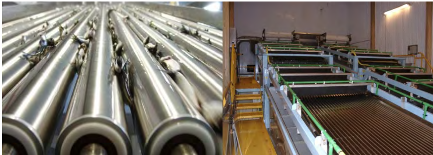
Figure 9. Rotating elements in grading machine and vibrating grading machine
