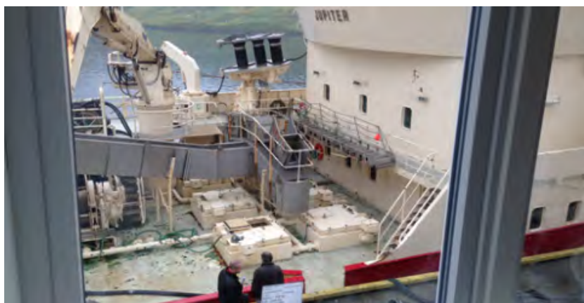
a) The boat with the catch has the fish in RSW water. After loading, the water is returned to the boat.
