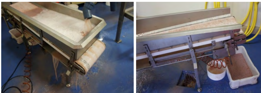
Figure 29. FiltreX – shrimp processing water filtration in Kampa
