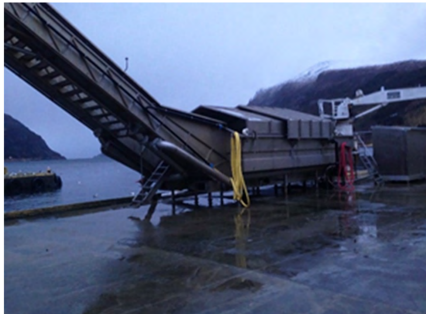
Figure 19. Fish is delivered by boat or trucks. The fish is kept in icy water and the water is after having processed the fish in the plant returned to the boat or truck. The recipient of treated wastewater is into the fjord which is seen behind the fish delivery station
