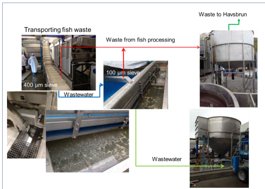
Figure 15. The waste is collected at the site. 400 µm sieves followed by 100 µm sieves are used underneath the transport conveyors. The water underneath is collected and treated in a flotation unit (DAF = Dissolves Air Flotation). The residual is delivered to Havsbrun for processing into fish fodder
