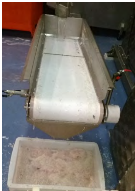
Figure 30. FiltreX – fish processing water filtration in H.G.
