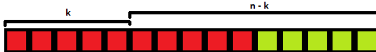
Figure 5.13: Errors which are corrected during step 4 for RS(15, 5) code. With the red color there are marked positions, where error can occur, and with green color are marked positions where error cannot occur.
