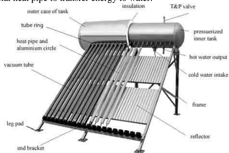
Figure 8-Evacuated tube solar collector (Greenterrafirma, 2013)
