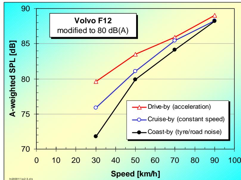
When vehicles are under acceleration, both tyre/road and power unit noise levels increase due to the extra tyre torque and engine load; the increases are normally the highest for power unit noise. This means that at such conditions power unit noise may occasionally exceed tyre/road noise on the 2<sup>nd</sup> gear (but hardly in higher gears).
