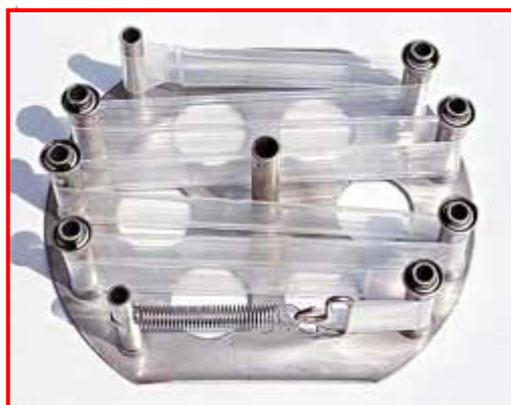
Figure 2.3 Spider carrier with mounted lipid filled membrane for SPMD sampling.
