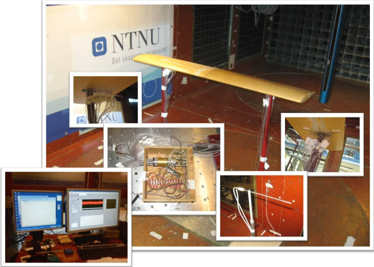
Figure 32 : Pressure Transducer and Data flow of from the Pressure Taps on the wing
