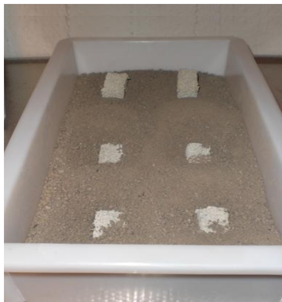
Figure 2. Arrangement of the sorbent material in the experimental box
