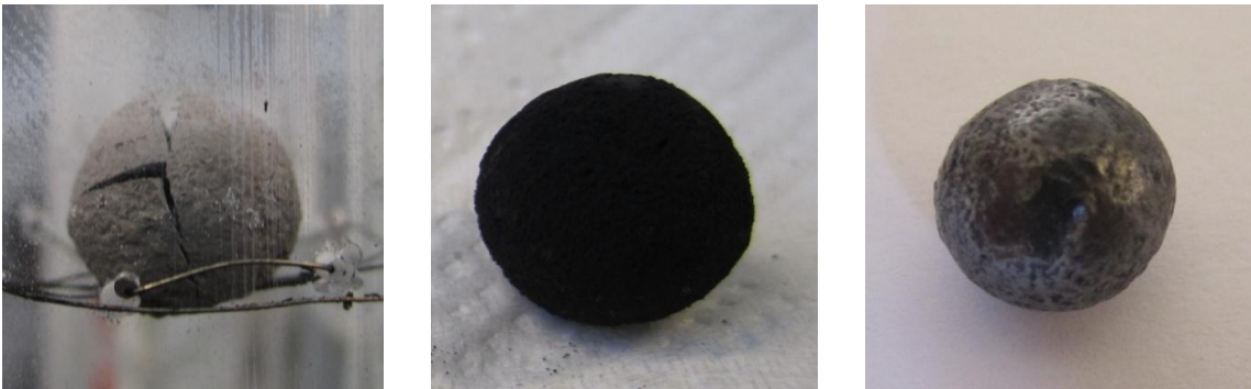
(a) Little carbon deposition. (b) Carbon deposition. (c) After carbon removal.
