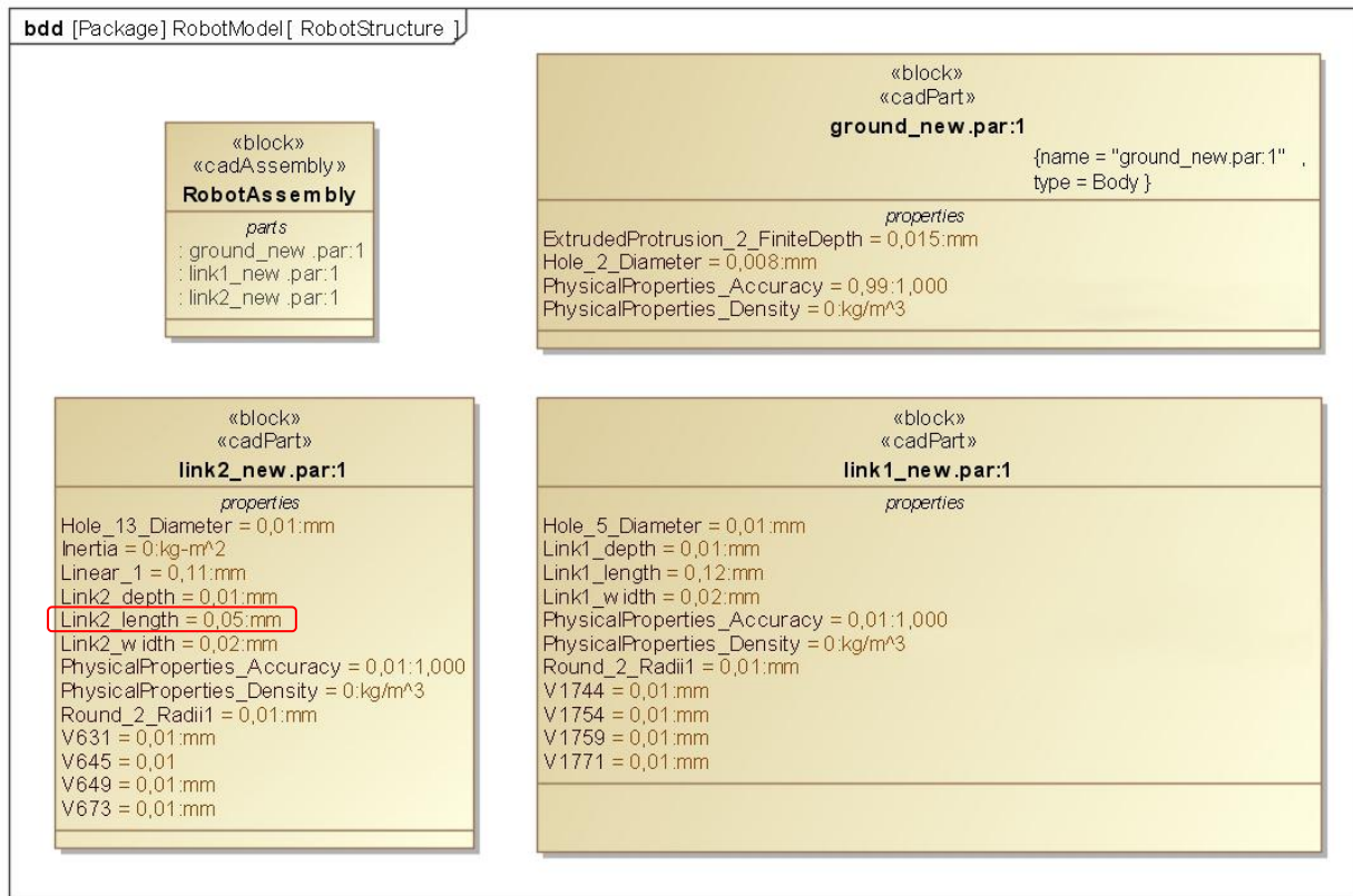
Figure 19 - Updated Robot Model in Magic-Draw
