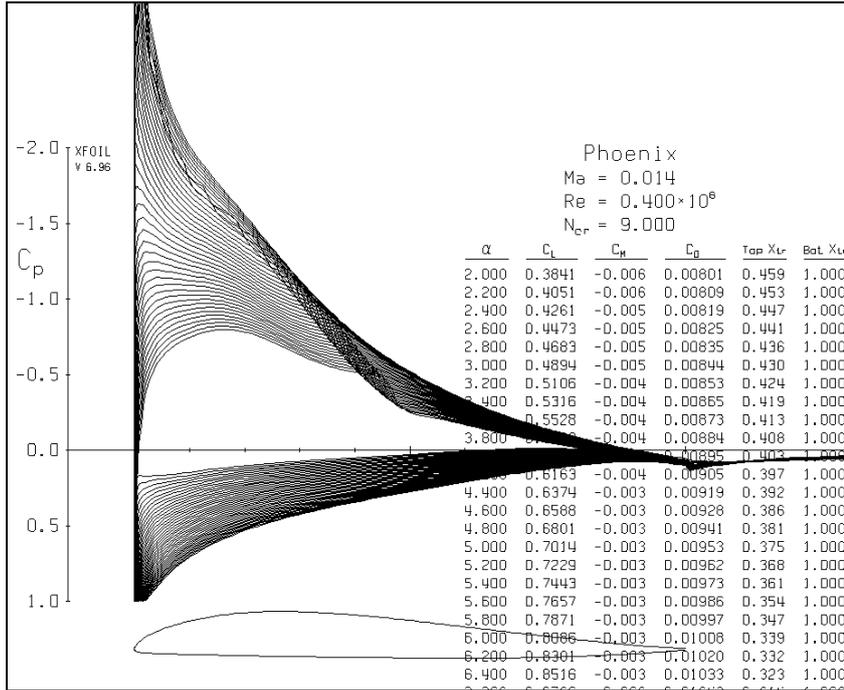
**Figure 8.** Example of how XFOIL displays a diagram of graphs, with a sequence of alphas where the calculations were successful.
