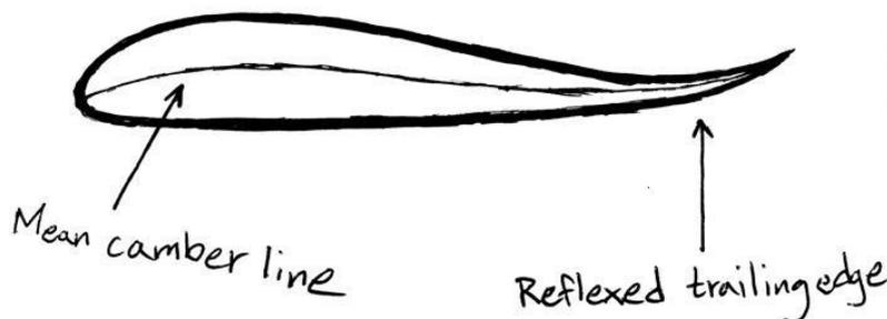
**Figure 2.** The image illustrates the typical characteristic shape of an airfoil with a reflexed trailing edge.
