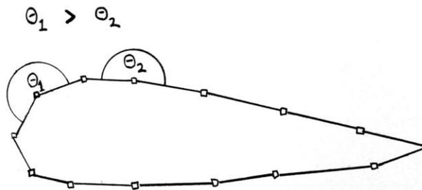
**Figure 6.** Illustration of how lack of nodes can create too big angles between the connecting lines.
