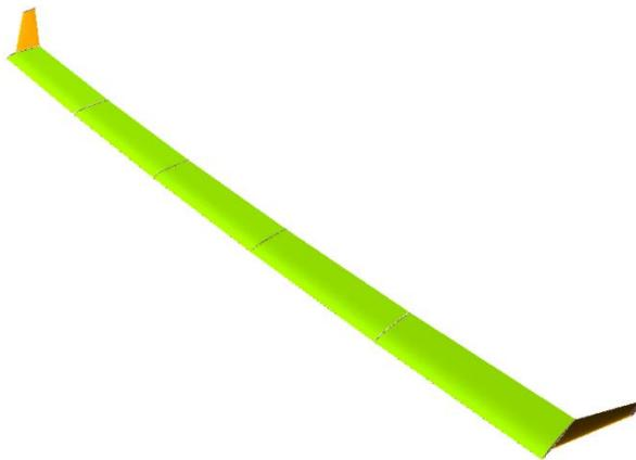
**Figure 1.** Example image of current but tentative design (five wing panel version). Motors on leading edge is not modeled. (Generated by Gustaf Enebog in SUMO).
