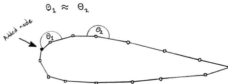
**Figure 7.** Illustration of how adding a node decreases the angle between the connecting lines.
