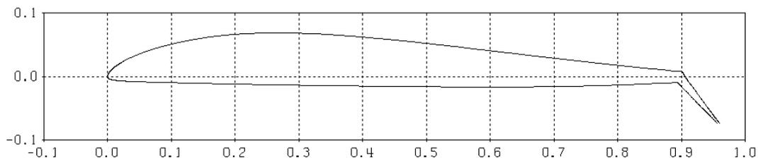
**Figure 15.** The 10% flap version of Phoenix at 50 degrees of flap deflection.
