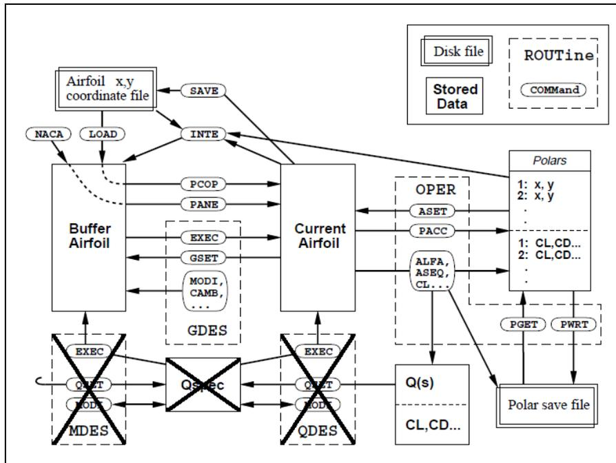
**Figure 5.** Illustration of the data flow in XFOIL. The menus marked with a cross are not used in the Solaris design method. The illustration was originally taken from "XFOIL 6.9 User guide, Mark Drela, MIT Aero and Astro. Harold Youngren, Aerocraft, Inc. 11 Jan 2001 (page 7)".
