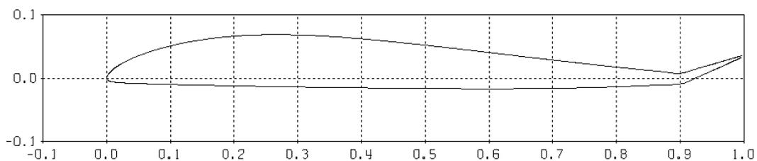
**Figure 14.** The 10% flap version of Phoenix at -20 degrees of flap deflection.
