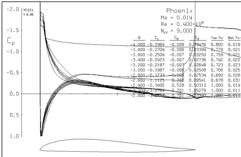
**Figure 9.** Example of how XFOIL displays a diagram of graphs, with a sequence of alphas where XFOIL fails to solve all the calculations. Many of the graphs look jagged and are quite irregular. The sequence is incomplete. XFOIL was only able to give the solution for -4 to -2 degrees in angle of attack, when the intention actually was to reach up to 10 degrees.
