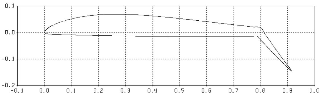
**Figure 17.** The 20% flap version of Phoenix at 50 degrees of flap deflection
