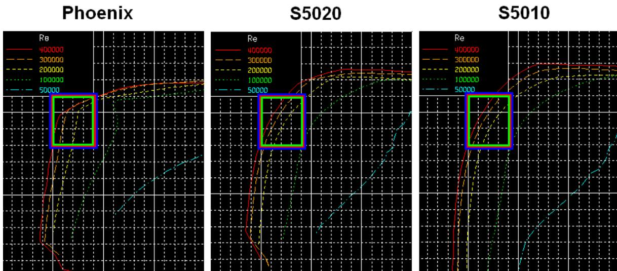
**Figure 12.**  $C_L$  vs  $C_D$  diagrams for the top three airfoils. By looking in the interesting area where maximum endurance is found (inside the multi-coloured square) it is clear that Phoenix is closer to the left, and because of that has a higher peak than the other two airfoils.
