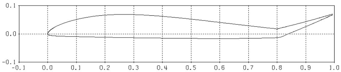
**Figure 16.** The 20% flap version of Phoenix at -20 degrees of flap deflection
