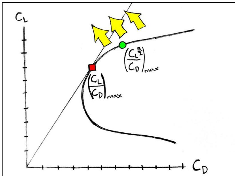
**Figure 3.** Illustration of how the ideal drag-curve should look like, when the aim is to maximize endurance.
