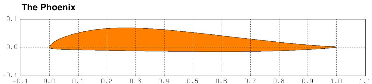
**Figure 13.** The geometric shape of the winner airfoil, the Phoenix.
