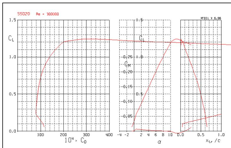
**Figure 10.** Example of how a graph is displayed inside XFOIL after using the PPLO command.
