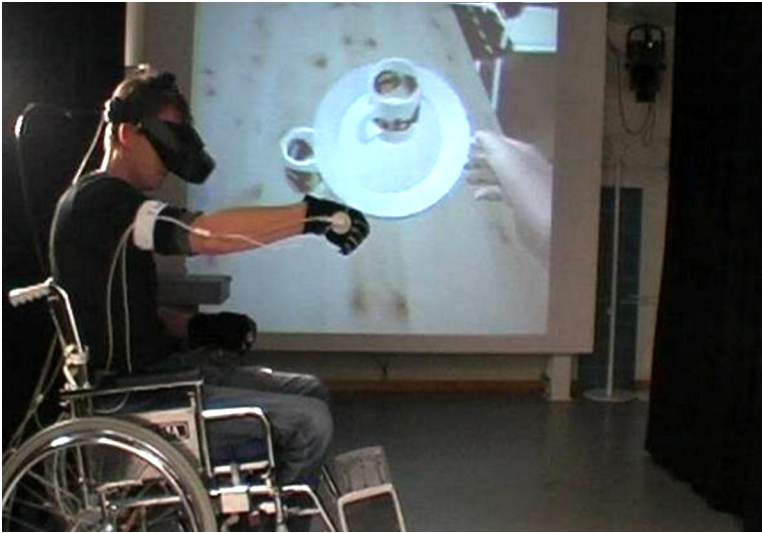
Figure 2.1: Classical full-fledged VR-setup with motion-tracked head-mounted display (HMD) and tracked, grip-sensitive, gloves. In this application the user can move around freely in the world by turning the wheels of the wheelchair. Hands are represented in the virtual world and can be used to grab and move objects with simulated physical properties. The head is motion-tracked in six degrees of freedom so that the user can look around freely by moving the head, e.g., to look under the table. This image is from an earlier VR-project in our lab.
