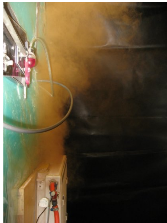
Figure 12. Illustrations from laboratory measurements. Upper left: warm side of the climate simulator where radiators were installed on the wall, together with a heater having integrated circulation pump, mass flow meter, and pressure controller; Upper right: cold side where ventilation air was taken in, measuring probes for airflow and temperature; Lower left: traditional radiator system where cold ventilation air (orange smoke) was brought in 1.5m above the radiator (no window); Lower right: ventilation radiator.
