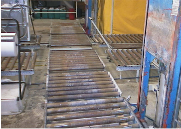
Figure 4. Roll conveyors for transporting appliances on between cleaning, high-voltage testing and new marking.
