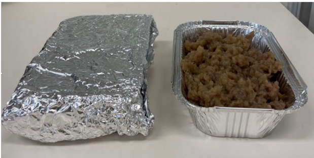
Figure 1: The drying procedure and heat treatment for pulps: the covered tray hindered water removal during heat treatment, whereas the open tray enabled drying.
