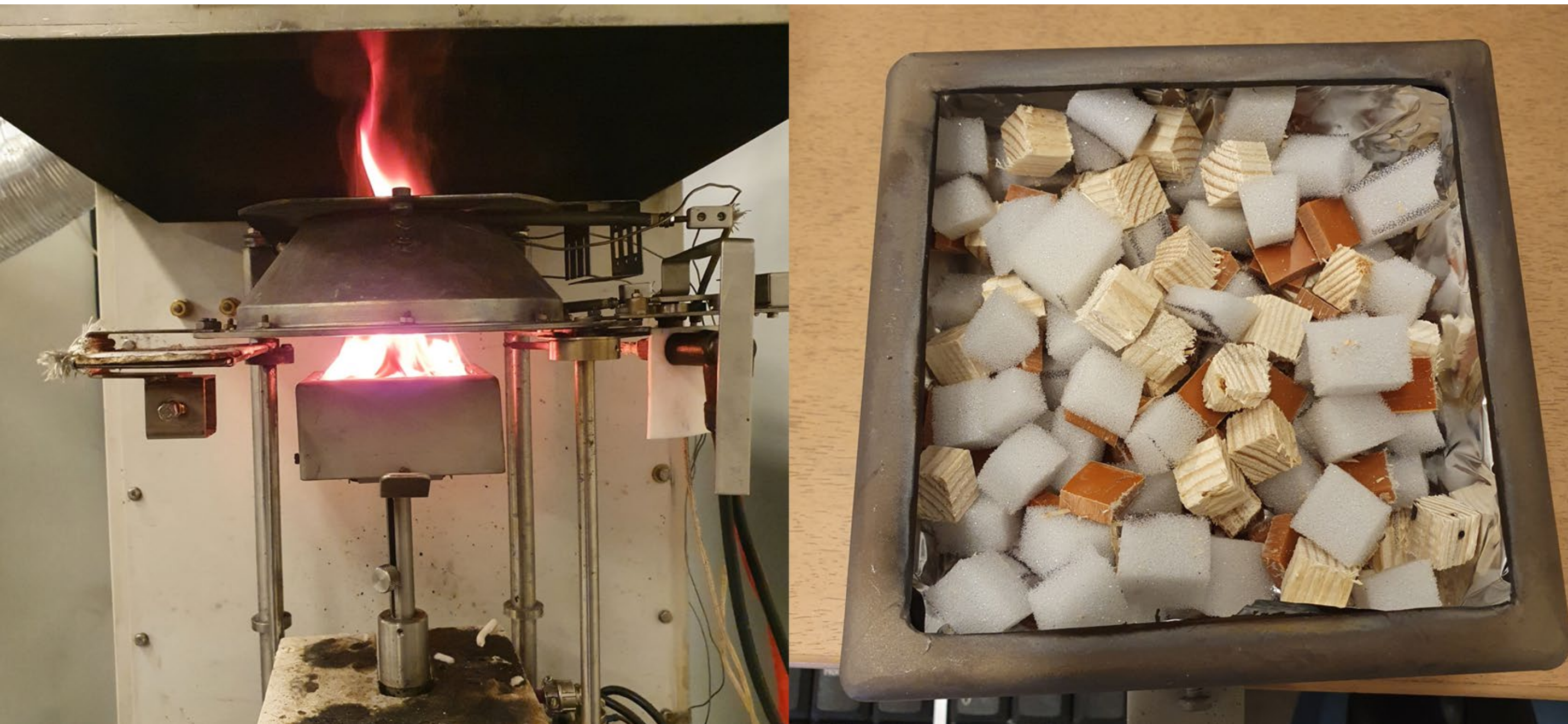
Generation of “standardised” smoke with the cone calorimeter according to ISO 5660 (right). Mixed cubic-shaped fuel consisting of wood, PVC plastic and foam mattress (left). Photo: RISE Fire Research
