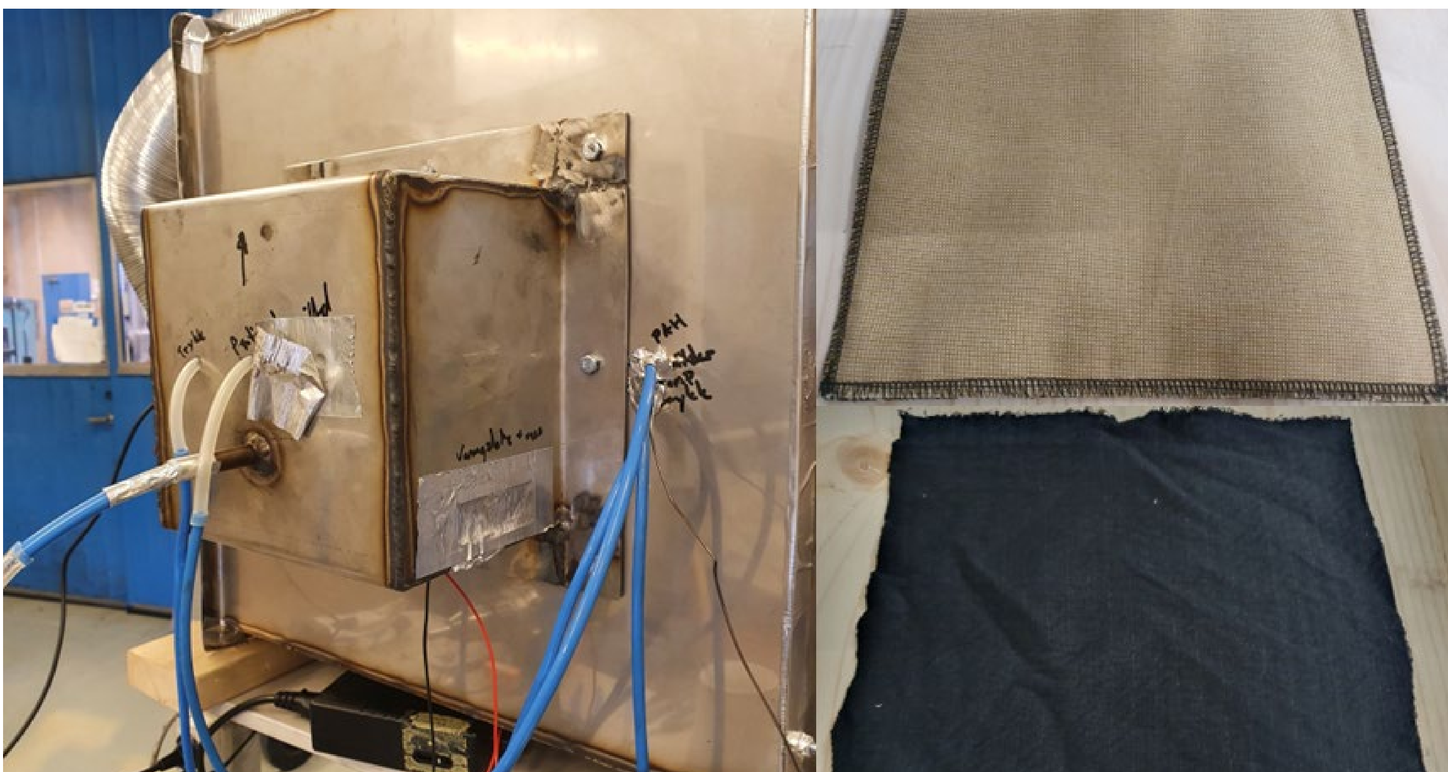
The exposure box where the textile specimen is positioned (left). The two different layers used in the experiment: PPE for firefighter (top) and wool undergarments (bottom). Photo: RISE Fire Research
