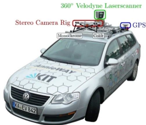
Figure 3.2: KITTI Recording Platform (Geiger et al. (2012))
