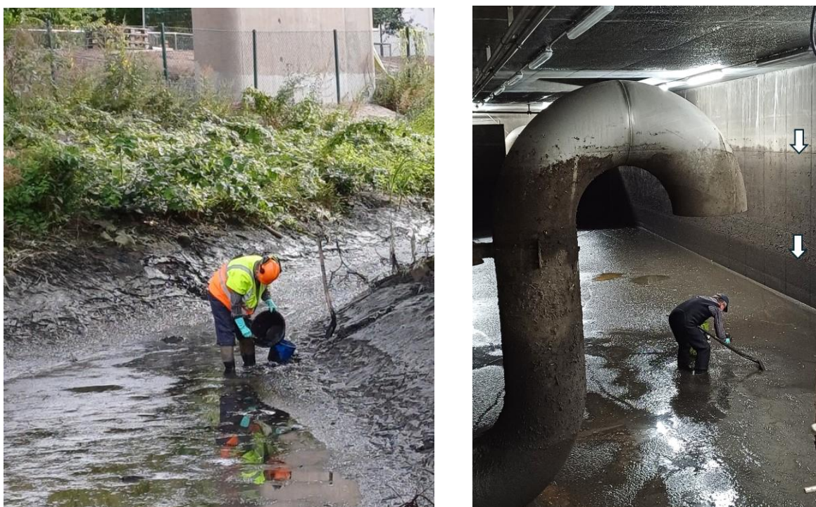
Figure 6: Left fig., Sediment sampling in the Lilla Essingen sedimentation pond. Right fig., sampling in the Gröndal underground treatment system. White arrows show high and low water levels in the sedimentation basin.
