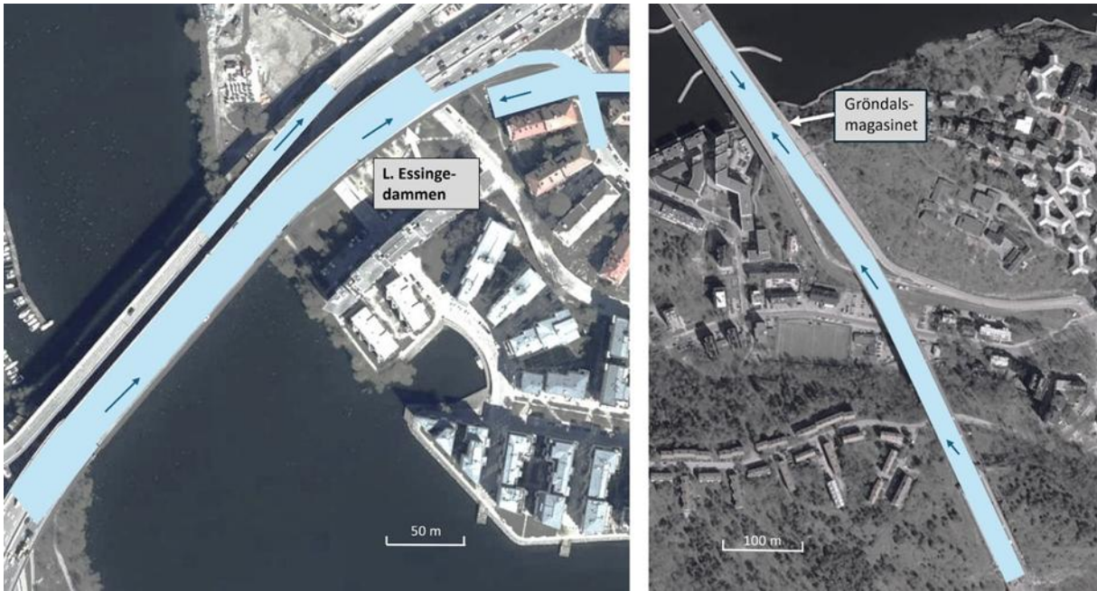
Figure 1: Catchment areas for Lilla Essingen RWTP (left) and Gröndal RWTP (right). Arrows showing the direction of runoff water to the runoff treatment plants. Maps based on https://kartor.eniro.se/m/1PJ1A .
