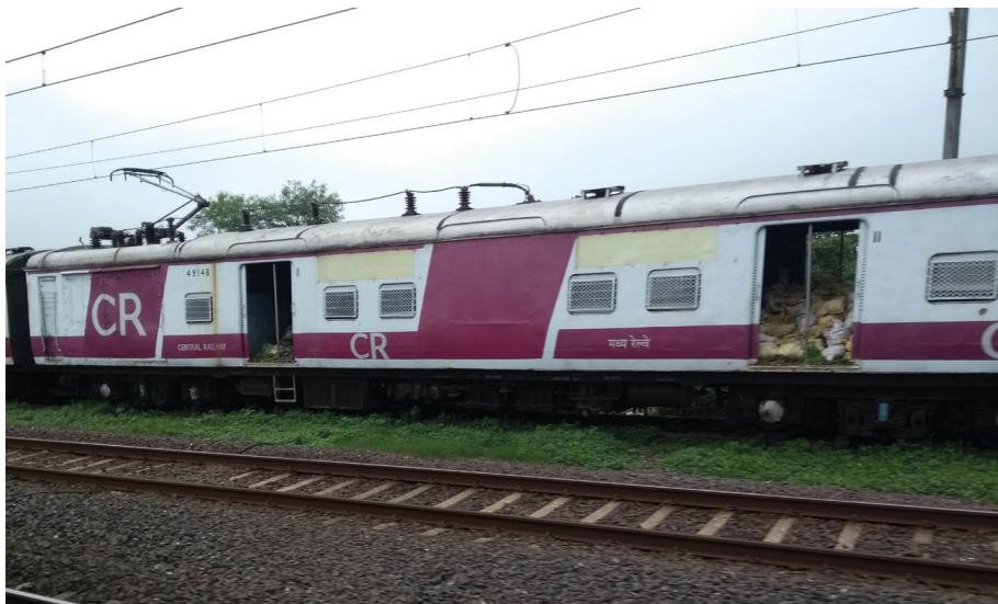
Figure 3: An AC/DC EMU rake carrying track debris.
