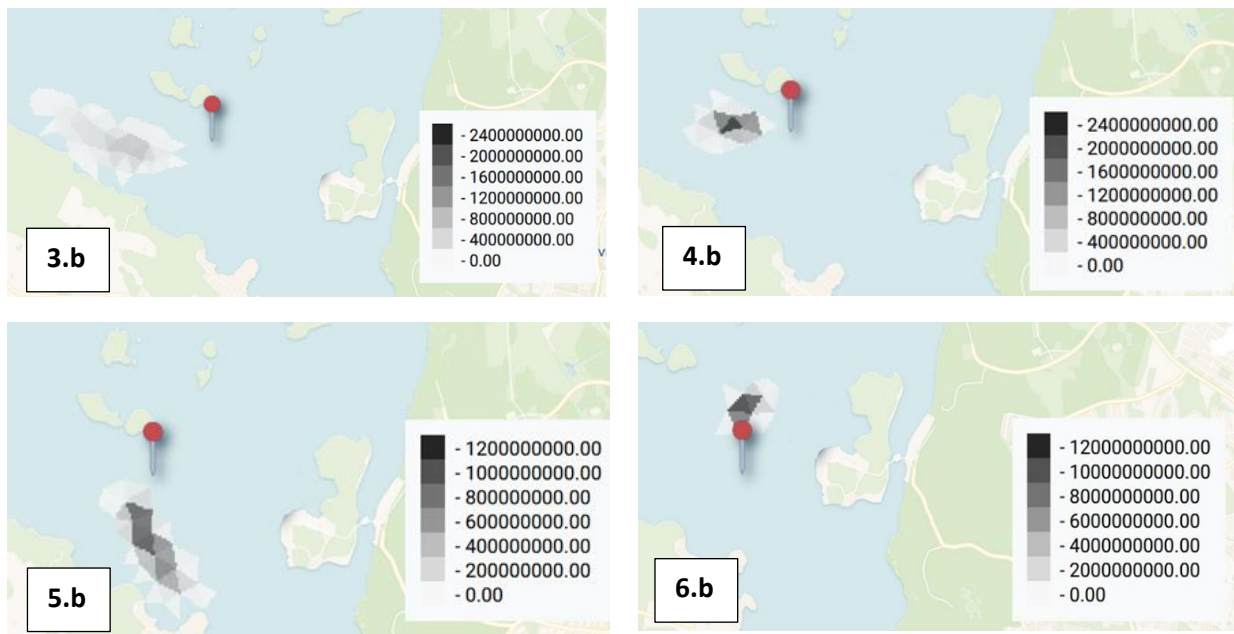
Figure 12. Visualizations of oil plume spreading using the DHI model for the six different simulation scenarios described in Table 4. Each visualization depicts the spatial distribution and movement of the oil plume over time. The water plant point has been removed from the visualizations for security reasons.
