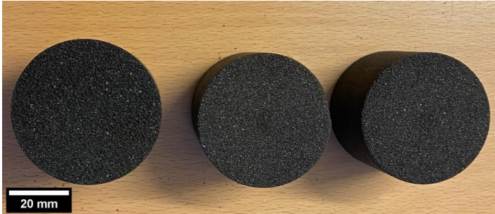
Figure 2.4 The cylindrical samples prepared according to DIN standards for permeability measurement.
