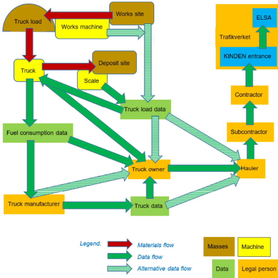
Figure F. Flow diagram example of fuel consumption information from transporting truck to ELSA.
