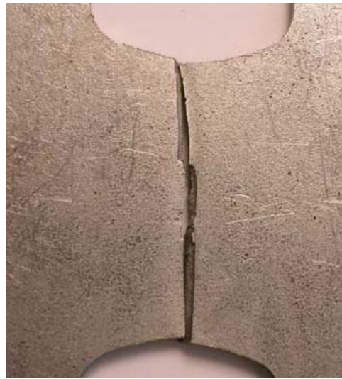
Figure 23: Real plane strain failure test of DP800. From [13]
