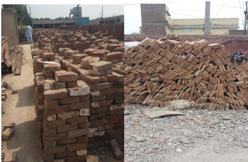
Figure 22 Reclaimed bricks after deconstruction process - Ref, Author.
