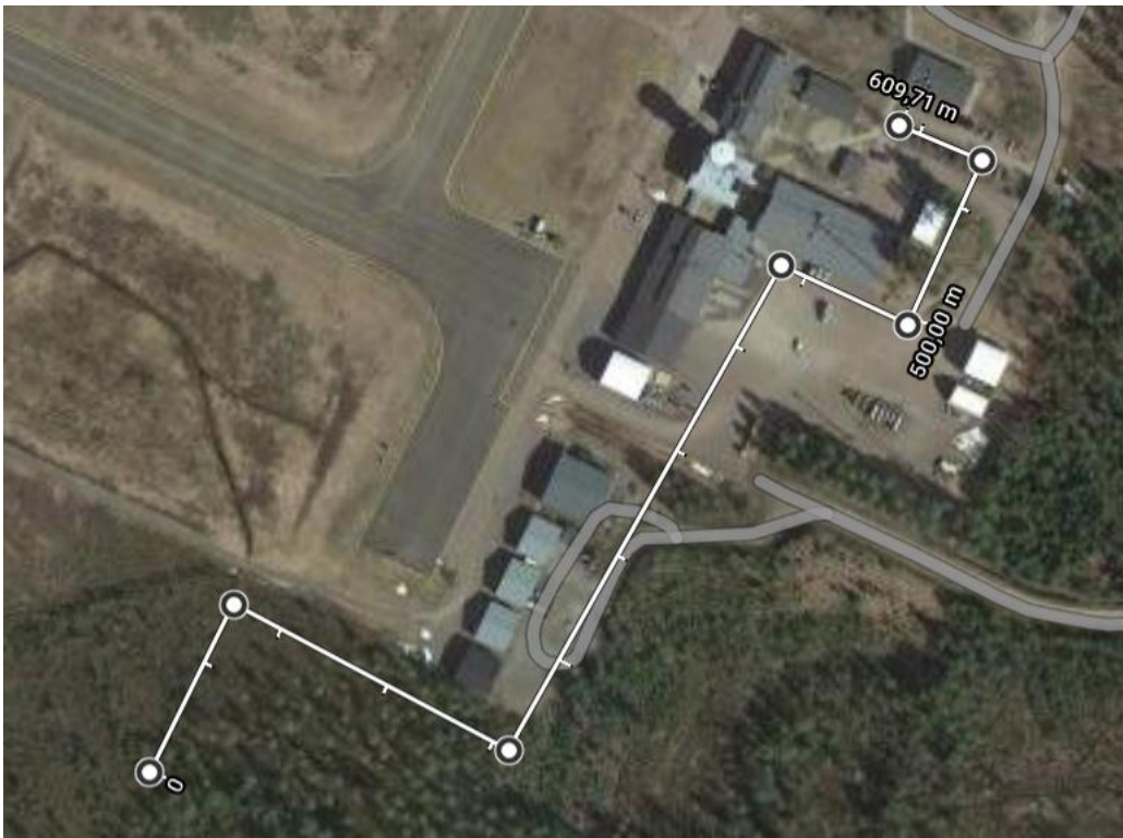
Figure 17: Sattelite picture of the facilities around the airport. The white lines are the suggested pathway for the transmission cables between facility and solar production.
