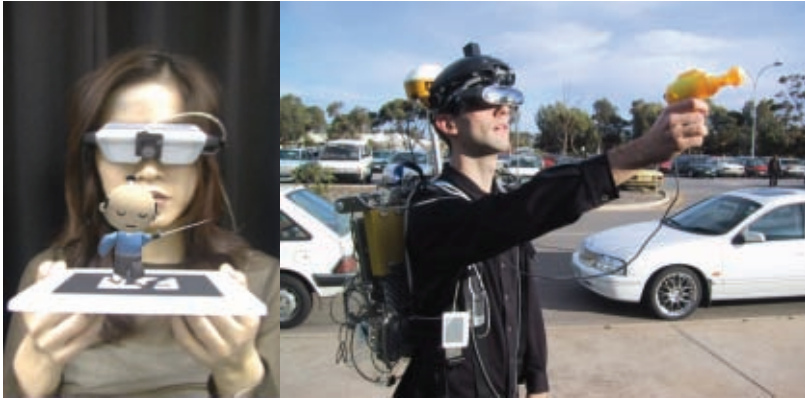
Figure 2.2: HMD in indoor and outdoor AR. Left image shows a HMD-based AR system with marker-based tracking and tangible interaction. Right image depicts Tinmith, an outdoor AR setup, used for playing AR Quake. In both cases, a commercially available opaque HMD has been made video see-through by aligning it with a camera. (Photographs courtesy of University of Washington and University of South Australia)
