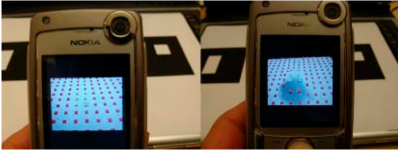
Figure 3.5: Selecting and manipulating several vertices to deform a polygon mesh. Selected vertices are locked to the phone and manipulated by phone movements. A group of vertices are selected by "painting" them and then framing one of them with the square located in the center of the screen.
