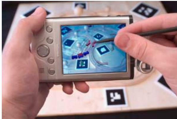
Figure 2.3: Handheld AR: Invisible Train. This application demonstrates marker-based tracking for video see-through AR on a PDA. Interaction is based on device motion for navigation and stylus input for selection and manipulation: in this case opening and closing track switches. (Courtesy of Vienna University of Technology.)
