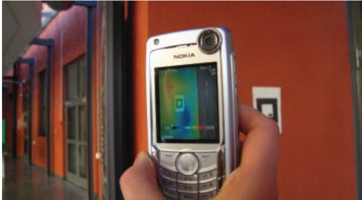
Figure 3.10: A concept where a mobile phone is used to visualize humidity data derived from an embedded sensor network was realized by placing sensors in a marker coordinate frame. This allowed a resulting live image to be registered with the element of interest.
