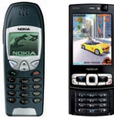
Figure 1.1: Phone evolution. The left phone is a Nokia 6210 announced in 2000. It has a monochrome display that renders 6 lines of characters. The right phone is a Nokia N95 8GB announced in 2007. It features a 2.8" TFT display with 16 million colors. It also has hardware 3D graphics acceleration and GPS positioning. On its back is a 5 megapixel camera and a second camera is located on its front. (Photograph courtesy of Nokia)
