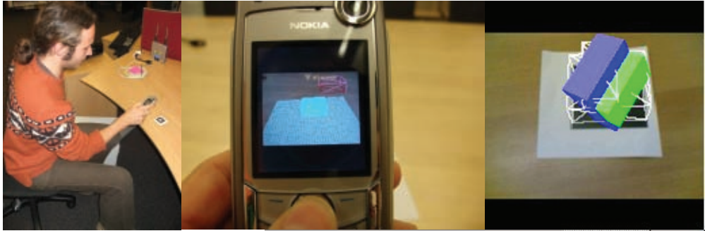
Figure 3.3: Experimental setup and tasks. Participants sat at a table with a tangible paper marker. In positioning and rotation tasks, they were supposed to align a solid block with a wireframe one as fast as possible.
