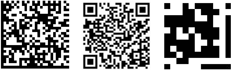
Figure 2.4: Data matrix formats. The left code is a SemaCode while the middle one is a QR Code. Both these codes encode the title of this thesis. The right code is a Visual Code that encodes the dissertation number of this thesis. All three codes have guidance bars and/or squares to identify corners and to facilitate both distortion correction and code scanning.
