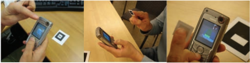
Figure 3.4: The left image shows 2D finger interaction based on motion field estimation. The remaining two show 3D finger tracking realized by putting a marker on one finger. In both cases, the front camera is used to register input.
