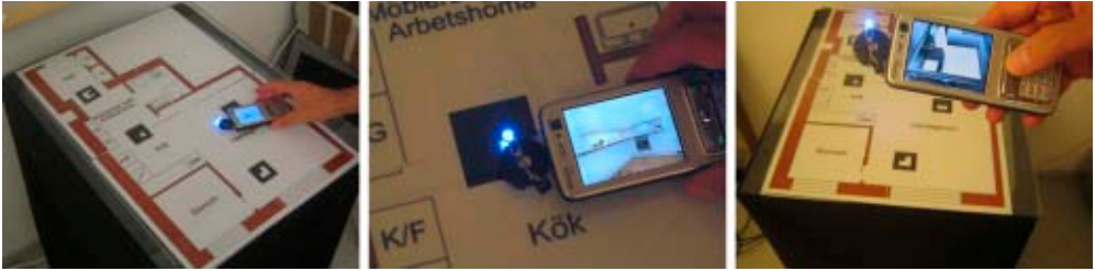
Figure 3.12: LUMAR: Merging three information spaces. Printed material (left) is augmented by 2D media (center) and 3D graphics (right). Moving the phone across the surface loads relevant images and lifting it makes a transition to 3D space. This example demonstrates how three different, but highly relevant, media can be merged into a single model of an apartment, browsed using device motion only.
