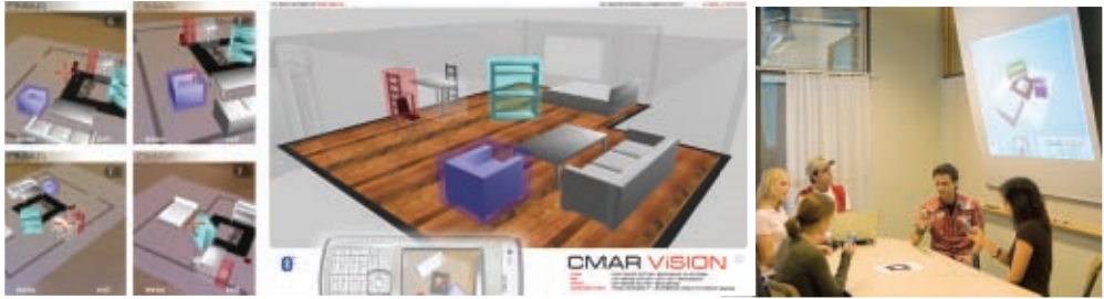
Figure 3.9: Four devices viewing and manipulating the same scene. CMAR ViSION, a PC client for high quality output on large displays. A group collaborating on furnishing an apartment.
