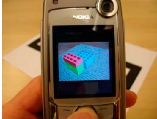
Figure 3.6: Virtual scene assembly using phone motion. Placing a crosshair and clicking a button allowed users to select pieces and manipulate them in 3D using phone motion. If the pieces were placed sufficiently close they were aligned and attached to each other.
