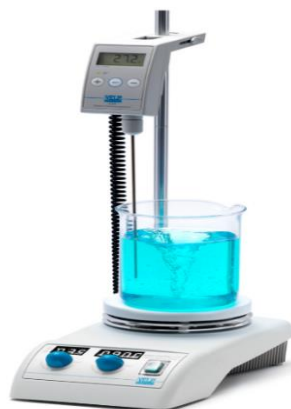
Figure 15. The magnetic heating stirrer used for acid washing [51].
