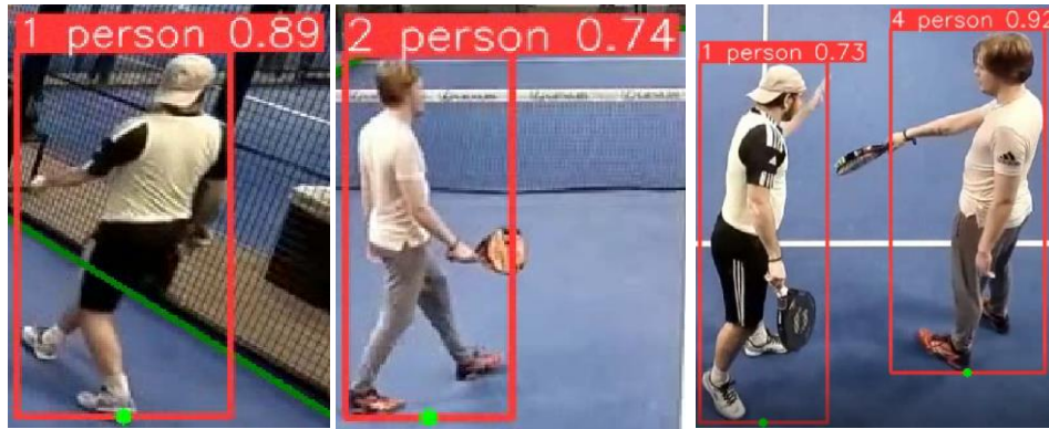
Figure 8, Object detection of the same players in two different scenarios. The first two images from left to right show two different players who have been detected. The right-most image shows the two previous players are in the same image. The bounding box represents where the person is believed to be. They are labeled with an ID, object class, and YOLOv5's confidence that they are this specific class represented by the decimal number.
