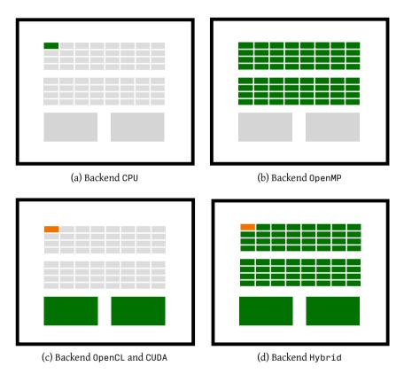
Figure 3.3: Node-level backends of SkePU.
