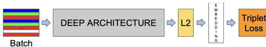
Figure 2.6 – Example model structure using triplet loss (Schroff et al., 2015)
