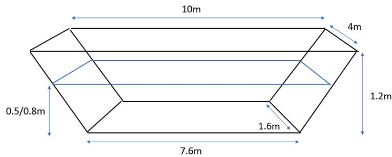
Figure 3: The wetlands were built to the above specifications.
