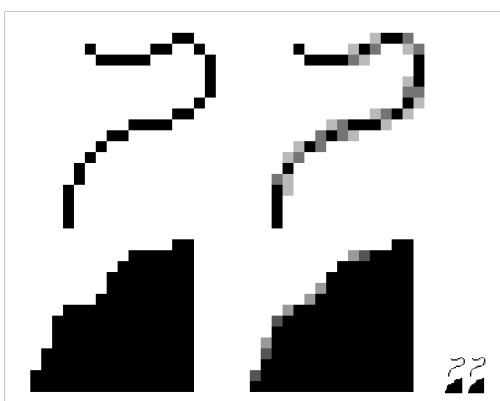
Figure 2 Example of how anti-aliasing smooths out a curve (Cure, 2010)
