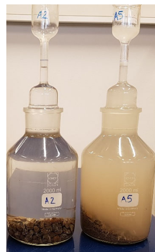
Figure 2.3 Aggregate water absorption using pycnometer
