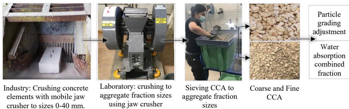
Figure 4.1 Production process of CCA for 50% and 100% CCA replacements
