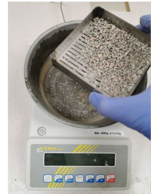
Figure 3.3 Flakiness of fine aggregates
