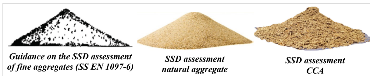
Figure 2.4 SSD assessment criteria for fine aggregates
