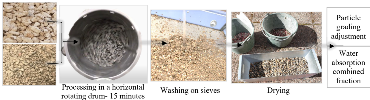
Figure 4.2 Mechanical pre-processing of CCA for 50% and 100% CCA replacements
