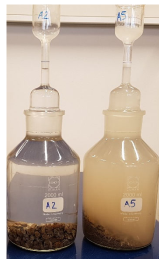
Figure 2.3 Aggregate water absorption using pycnometer
