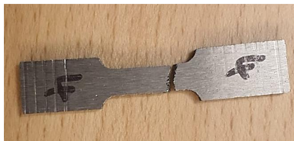
Figure 39: Sample after tensile testing.
