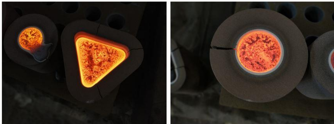
Figure 20: Cracks Generated in Molds
