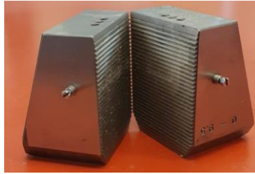
Figure 40: The groove wedge used to hold the samples in grip
