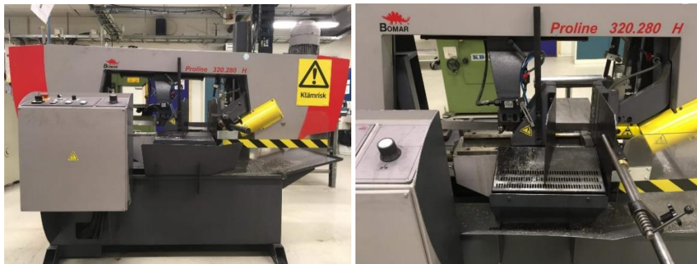
Figure 22: Proline 320.280H semiautomatic bandsaw used to cut the cylinders for the thermal and tensile tests
