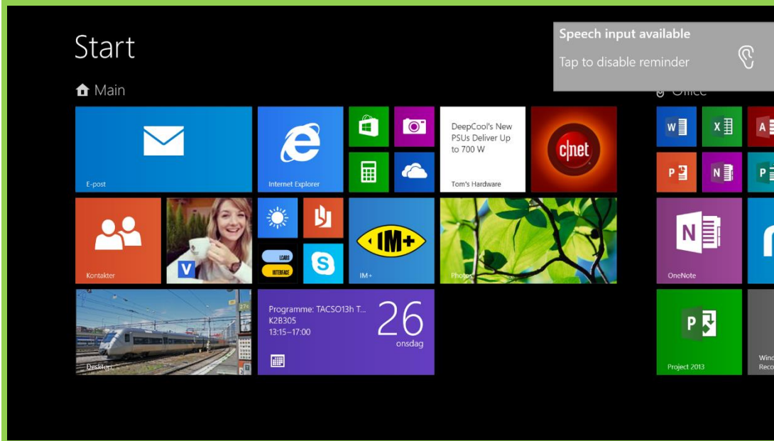
Illustration 6: Voice activated Windows 8 UI using a toast to present a speech input modality.
