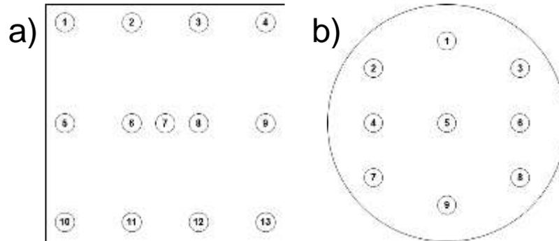
*Figure 18* Points of measurement for determination of film thickness with numbers showing the order of measurement for samples made by (a) handsheet forming (a) and (b) vacuum filtration
