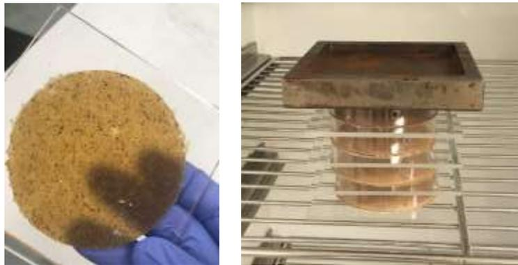
*Figure 17 Biomass film adhering to acrylic sheet after pressing (left), stack of biomass films in drying setup with weight on top (right)*
