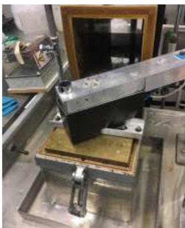
*Figure 13 Pneumatic press on top of the wire screen to remove water from wet-laid films*
