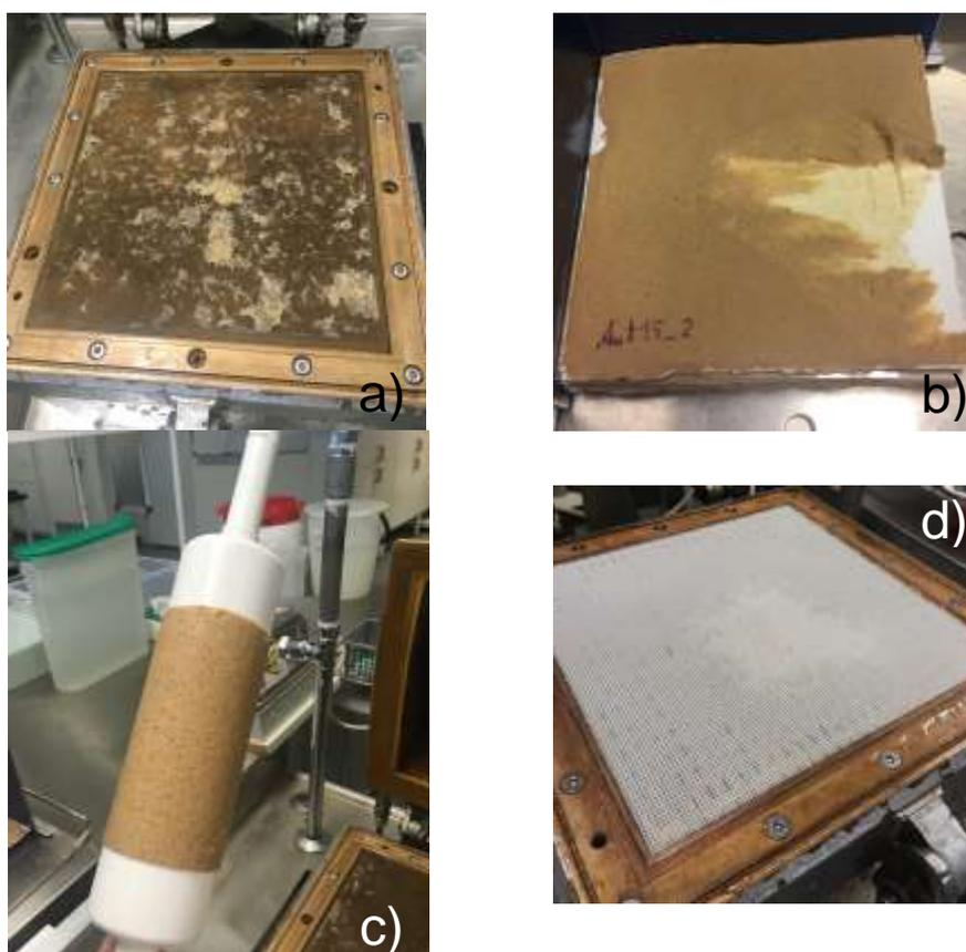
*Figure 12 Biomass residue on phosphorous bronze wire screen (a), damaged biomass film due to sticking to wire screen (b), biomass film attached to pin roll for damage-free recovery (c), nylon wire screen without major biomass residue (d)*
