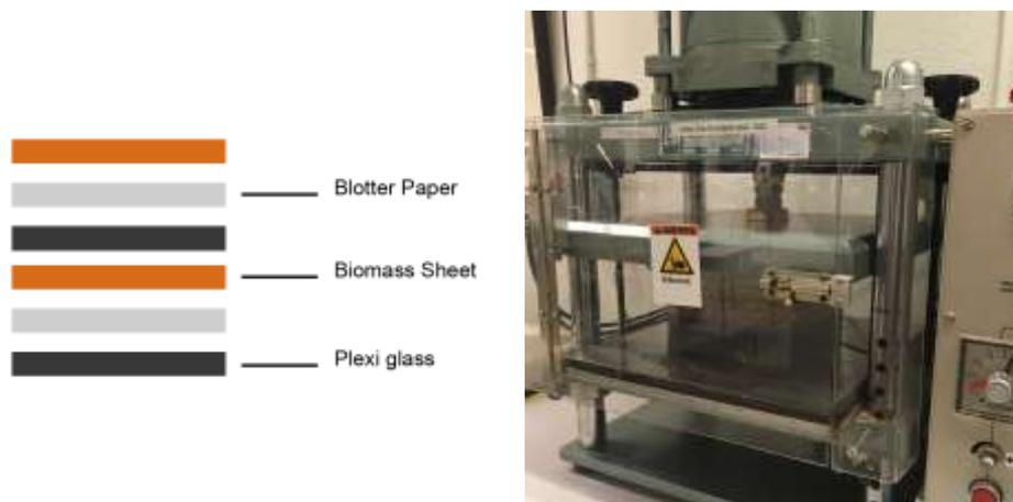
*Figure 14 Schematic of stacking order of wet-laid films (left), stack of films in hydraulic press at 0.395 MPa for 7.5 minutes in total (right)*
