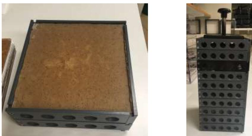
*Figure 15 Wet-laid film after pressing mounted in drying rack (left), stacked drying rack with weight on top for fixation (right)*
