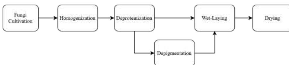
*Figure 6 Schematic process of film preparation from fungi*
