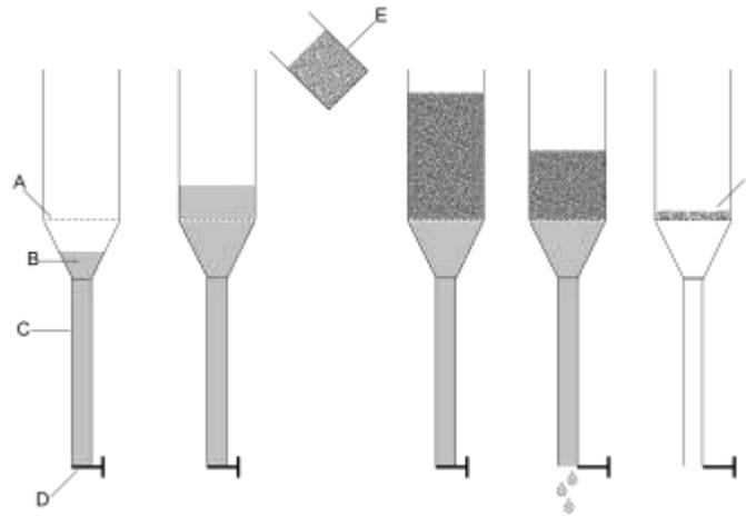
*Figure 5 Schematic of the wet-laid process using a handsheet former. The column is first filled with water till above the wire screen. Then a fiber-water suspension is added. Drainage is started after the suspension has been agitated. A wet-laid web remains on the wire screen*
