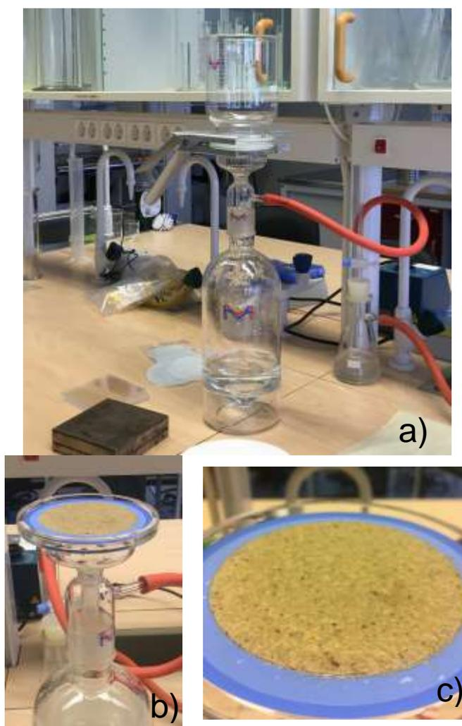
*Figure 16* Full vacuum filtration setup with glass funnel clamped to the screen holder and flask (a), biomass film collected on nylon screen (b), close-up of biomass film on screen (c)
