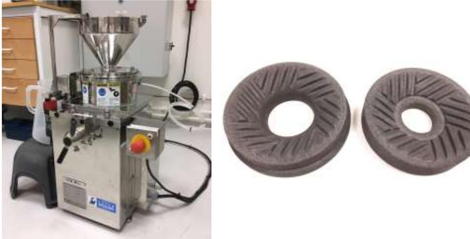
Figure 10 Disc mill grinder with feeding funnel on top (left), dismantled grinding disc pair (right)
