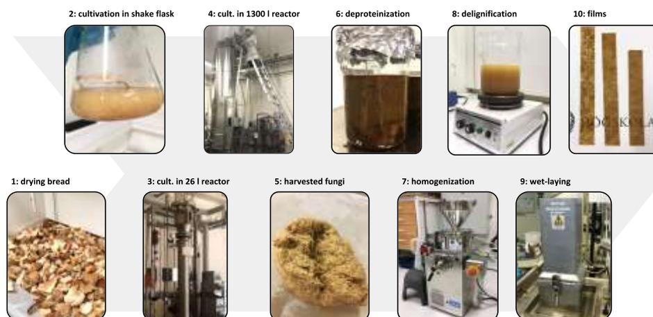
Figure 7 Method for film preparation from filamentous fungi
