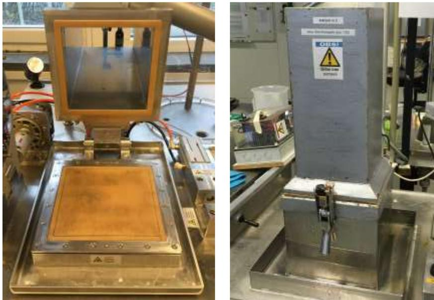
*Figure 11 Open handsheet former with phosphorous bronze wire screen installed (left) and closed handsheet former with a capacity above the wire screen of ca. 10 l (right)*
