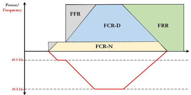
Fig. 2. Frequency restoration process, adapted from [17]
