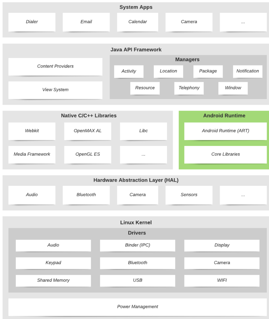
Figure 2.1: Android architecture, illustrated as in Google’s Android documentation [5].
