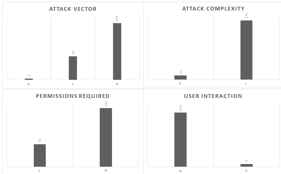
Figure 4.6: Frequency chart of the Exploitability Metrics for the 183 vulnerabilities for Qualcomm's Snapdragon Chipset from NVD.
