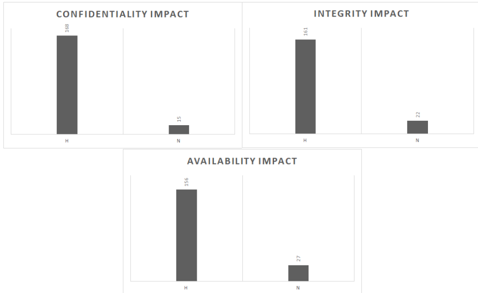
Figure 4.7: Frequency charts of the Impact Metrics for the Qualcomm Snapdragon 802A chipset.
