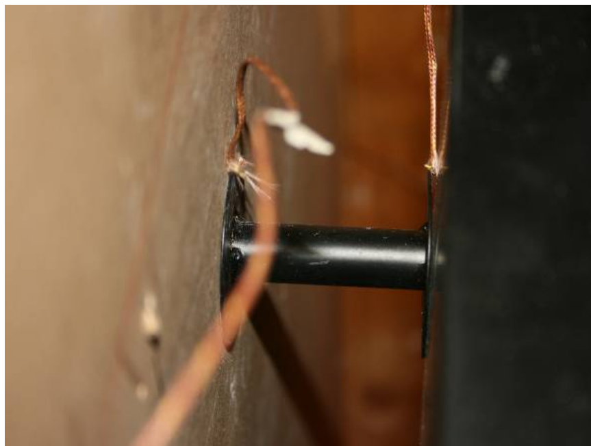
Figure 6-3 The temperature was measured in both ends of the distance piece. The distance pieces were installed with screws from the inside of the burning chamber.
