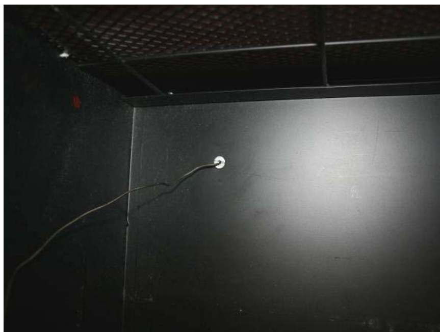
Figure 6-4 A hole was drilled on the head of the screw so that the temperature was measured 20 mm further inside the screw. The temperature was measured to be 92 °C.
