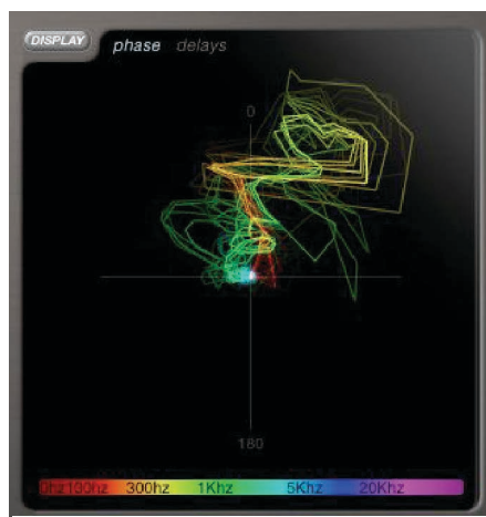
Figure 4. Auto-Align features a phase scope with detailed information on phase and frequency relationships.
