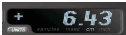
Figure 5. Auto-Align distance indicator allows us to estimate the distance in the computer and check for better phase relationships.
