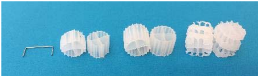
Figure 11. Different kinds of carrier material used in the study; K1H (AnoxKaldnes, Veolia Water Technologies), YL-1 (Jiangsu Yulong, China) and HXF12KLL (Stöhr, Germany). A staple (12 x 6 mm) is used as a size reference.
