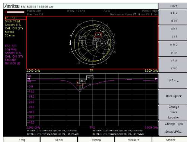
Figure 4.11: Measured S_{11} parameters of the Normal Patch Antenna.
