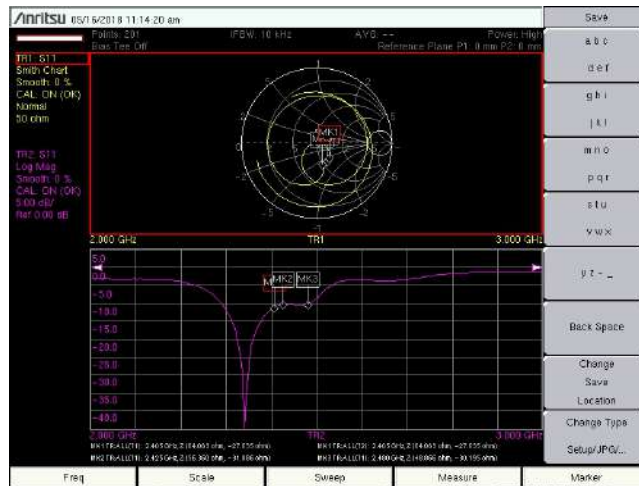
Figure 4.6: S_{11} parameters of the Manufactured Square Ring Meandered Antenna.
