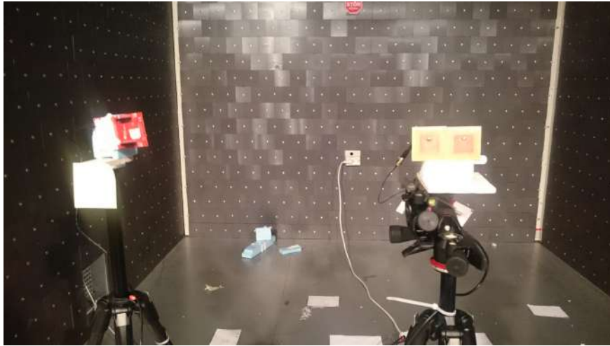
Figure 6.19: Test setup of SPA antennas.
