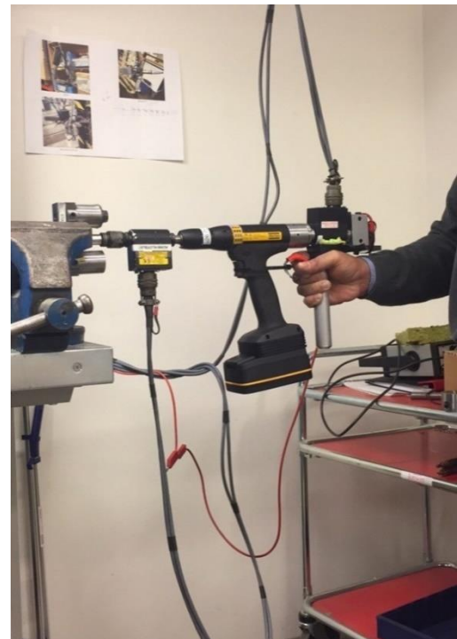
Figure 20. The experiment setup with joints, sensors and simulated tool handle (vertical workspace).
