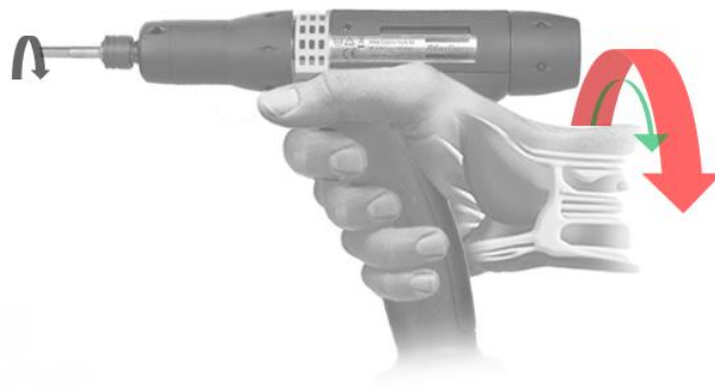
Figure 11. Motion of wrist when exposed to reaction torque during pistol grip power tool use. (5)
