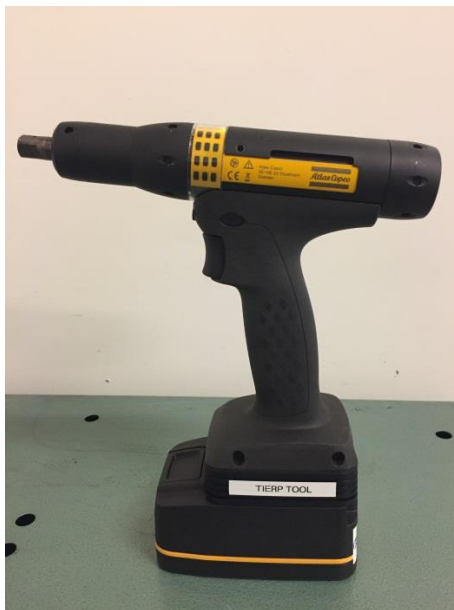
Figure 15. The electrical pistol grip nutrunner used in the experiments.
