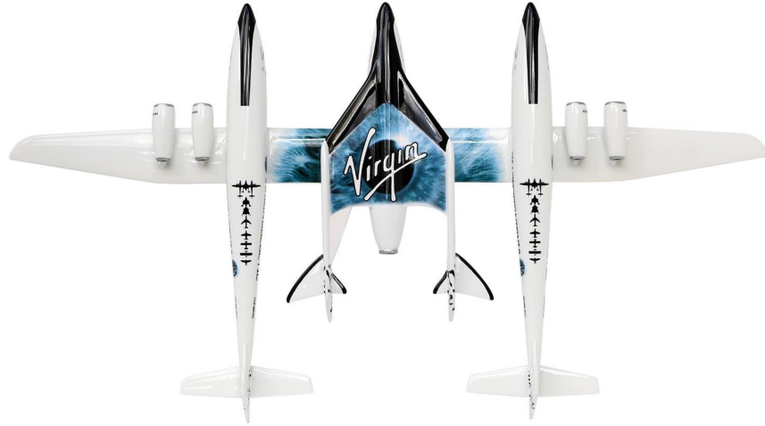
Figure 4.3: Model of “Space Ship Two” mounted to the mothership “White Knight Two” as seen from below[62]
