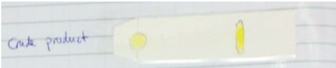
Figure 9. TLC analysis of FITC- \alpha -Lys-D70 ( R_f = 0 ), showing presence of free (FITC) _2 -Lysine ( R_f = 1 ).
