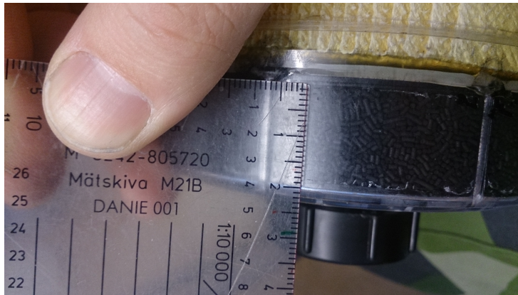
Figure 3.1: Measurement of height of activated carbon part of Skyddsfilter 90.
